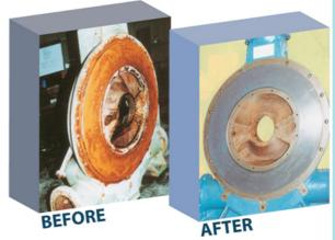
This system ensures minimal disruption to production for the cost of a repair rather than the cost of a replacement pump. Our 'service exchange' pumps are fully guaranteed and are protected with our high quality 'ceramic' coatings which ensure a service life longer than a new, unprotected unit.
