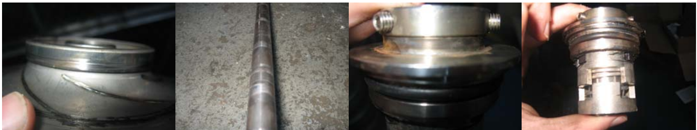
Light wear to impeller
