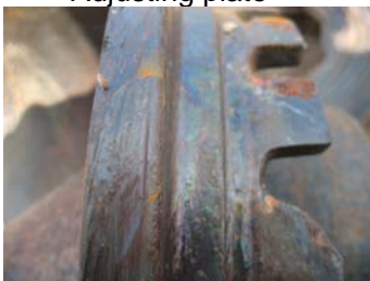
Wear to impller OD and back face
