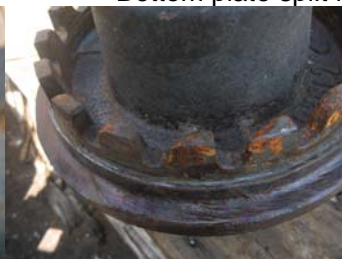
Wear to impller OD and back face
