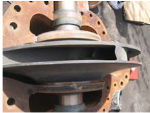
Impeller vanes and shrouds
