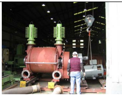
FLOWTECH 6000 C/W GEAR BOX PERFORMANCE TEST AT MANUFACTURER (NEW SUPPLY)
