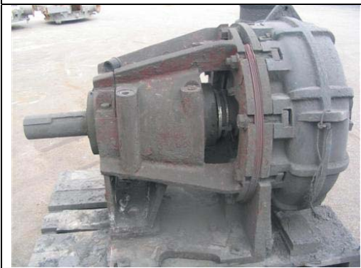
METSO MINERALS/SVEDALA/ DENVER COMPONENTS RECOVERED WITH BELZONA 1812 CARBIDE COATING
