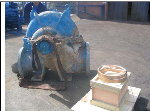
SPP SPLIT CASE - COATED WITH BELZONA 1341 ENERGY EFFICIENT SUPERMETALGLIDE
