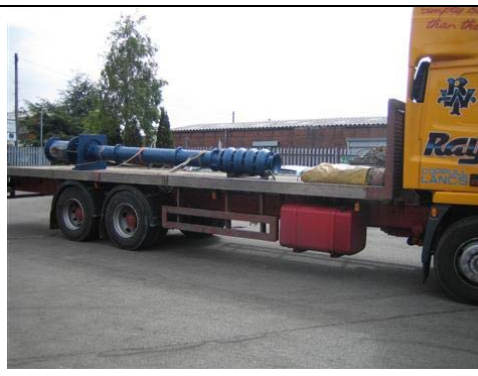
MATHER & PLATT VERTICAL AXIAL FLOW COATED WITH BELZONA
