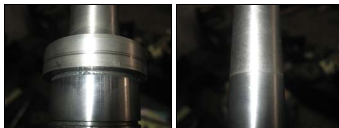
Worn locations on shaft
