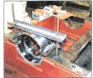
RESEAT LOOSE BEARINGS
